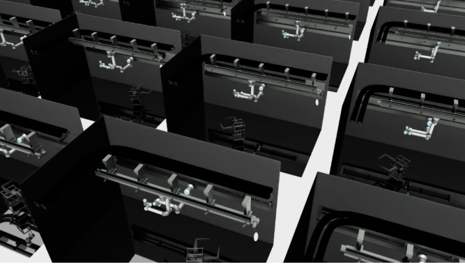
Fig. 11: PINGU digital twin in the Space Robotics Bench. Thousands of parallelized copies of the laboratory environment running simultaneously on a single GPU inside IsaacLab. Each instance contains a full PINGU model (air-bearing platform with two LEVION arms) and two UR10 manipulator mounted to the ceiling and wall rails, replicating the physical laboratory layout. Massively parallel rollouts with domain randomization enable the sim-to-real transfer results reported in Section IV.
